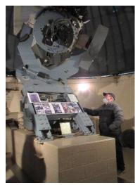
The tour continued to the Martz dome, which houses a 24-inch Dall-Kirkham telescope with a 16-inch RC Ritchey-Chretien wide field telescope attached to it. These are fully autonomous scopes that can be remotely controlled from the observatory control room and off site.
